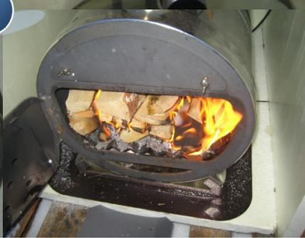
**NOTE!** Completely open air draft setting as shown in picture 4 gives an even better draft, but at the same time higher smoke temperatures.
